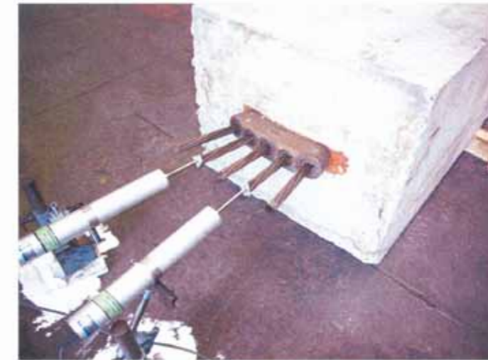
Figure 2 Setting the dial gauges to measure elongation of the wire strand.
