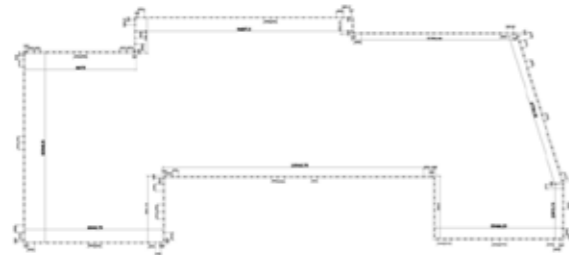
Location of Ground Anchors Around Periphery of Diaphragm Wall
