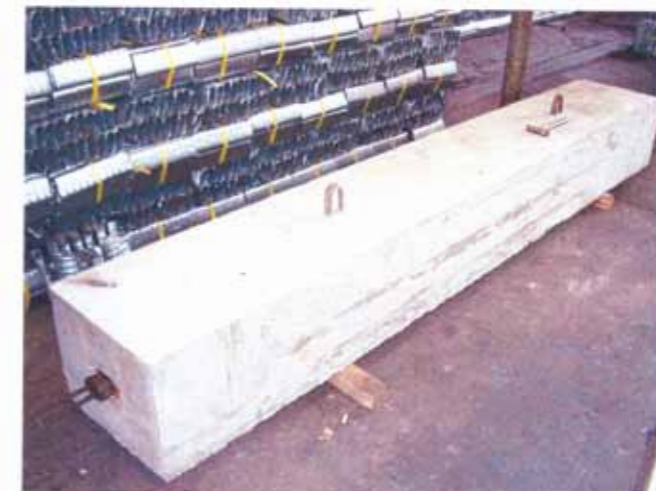
Figure 1 Test of load efficiency and of elongation of the anchored tendon
